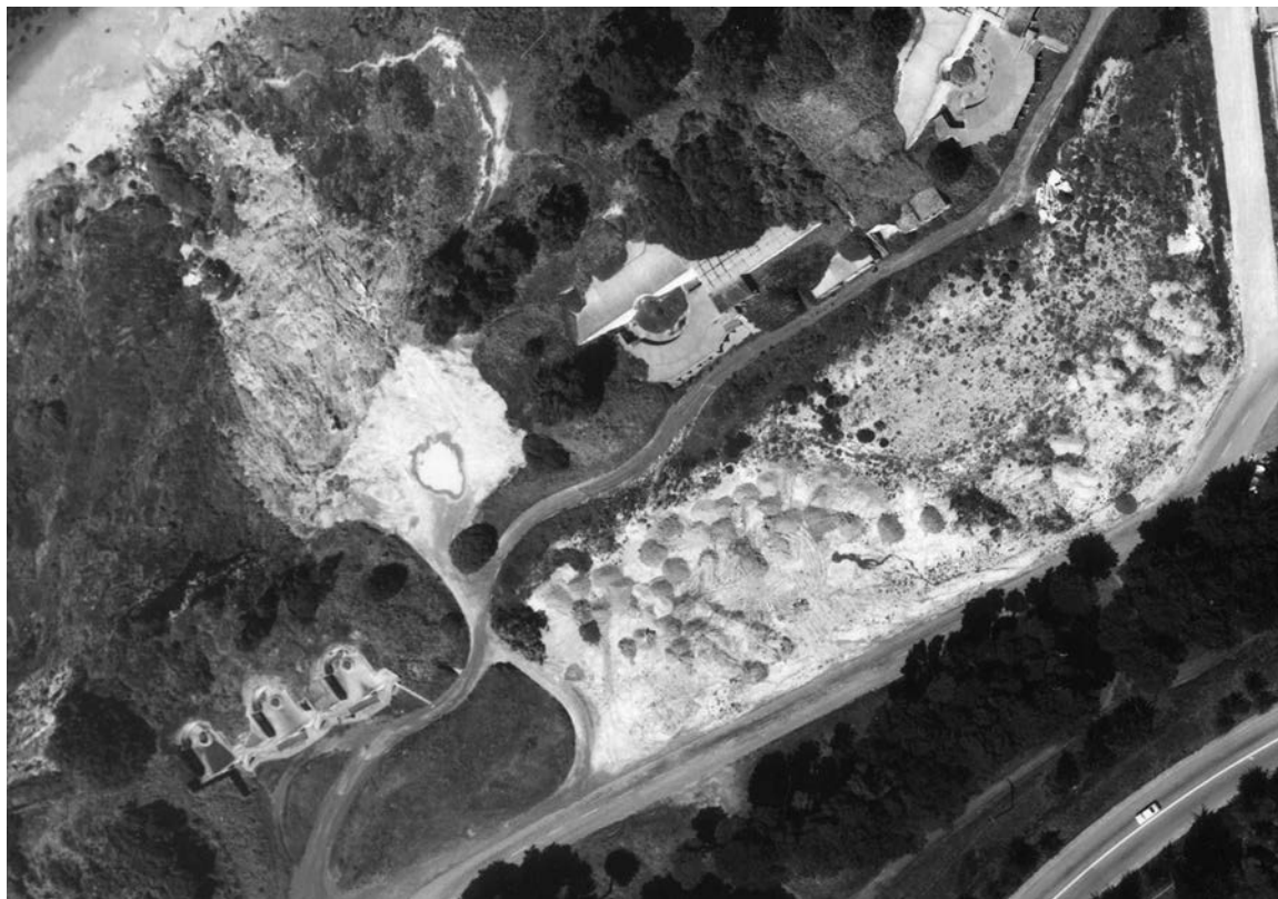
Fig. 28. Aerial photo taken in May 1967 documents extensive fill on the former site of both the dump and across the road behind the batteries. A pool of water has apparently formed directly over the dump site. The curved outlines of the traverses flanking the former battery are still visible.
