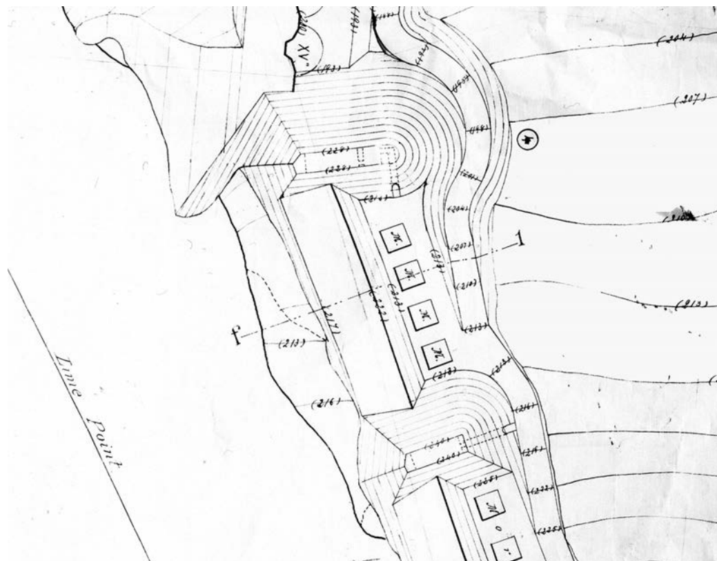
Fig. 20. Section of original 1870 engineer plan showing Traverses 21 (top) and 22 (bottom) and positions for 13-inch mortars. NARA, RG 77, Dr. 94, Sht. 102.
