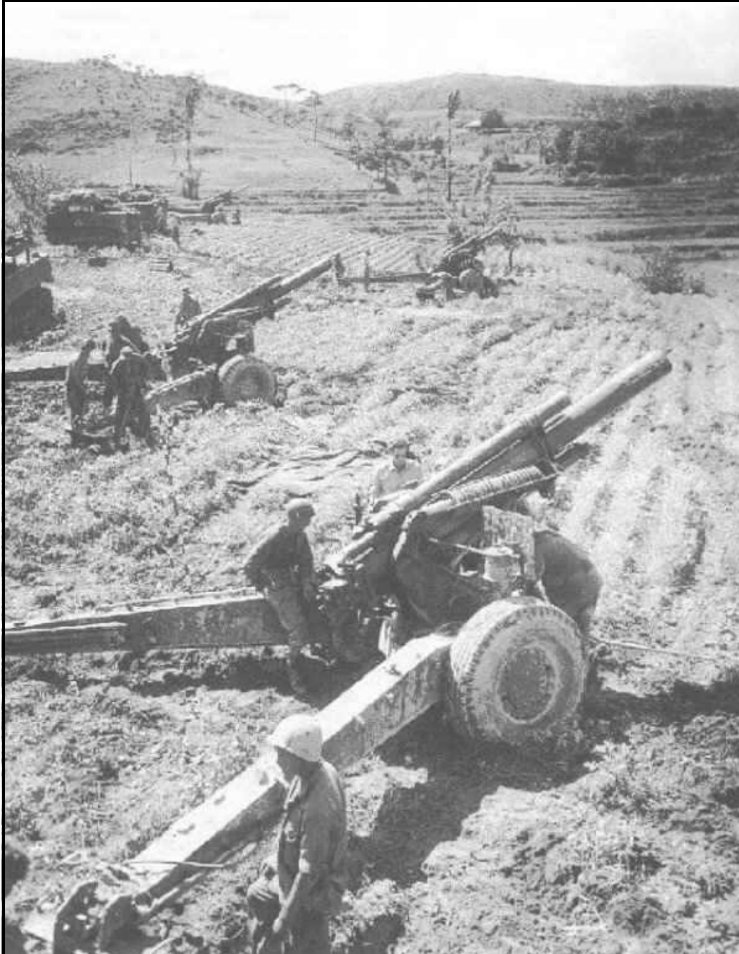
Tractor-drawn, 155mm howitzers of the type used by the 981st Field Artillery Battalion in Korea.
