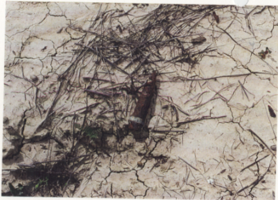
J-7 A 20mm target practice (TP) projectile found on the air to ground target range
