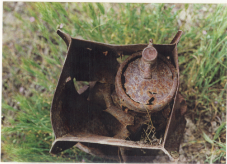
J-4 A fin assembly and spotting charge assembly from an M38A2 100-LB practice bomb
