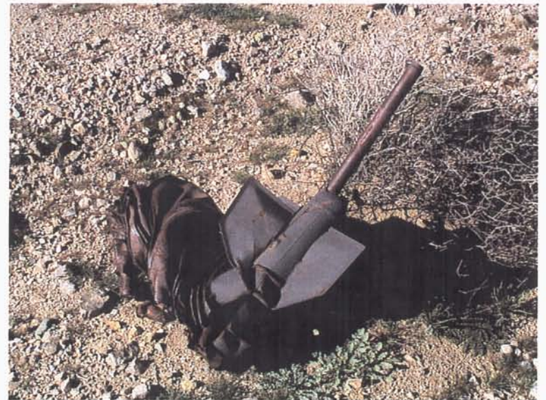
J-8 Looking at one of the two M124 250lbs. Practice bombs found on PBR #14 near the #3 target ring in Area A.
