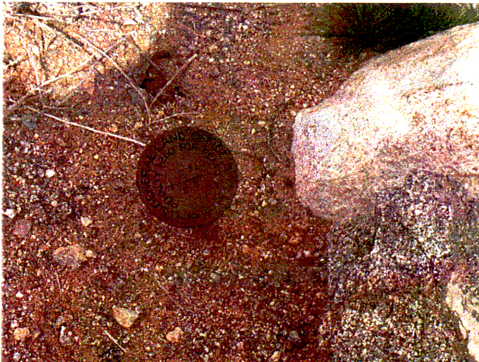
J-8 Survey marker which designates the exact location of this former target area
