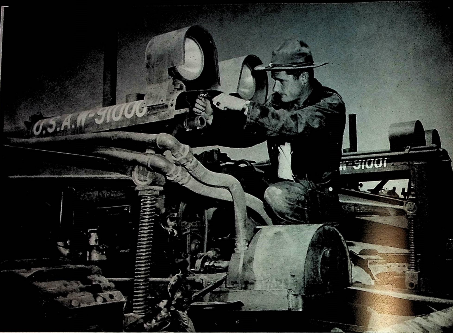
RADIATOR ON BULLDOZER IS REPAIRED BY A 115TH ENGINEER
